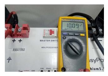
Using a multimeter, there should be and idling voltage of 10V
