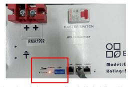
Illustration above shows how the battery would probably look like, with a red alarm LED ON
